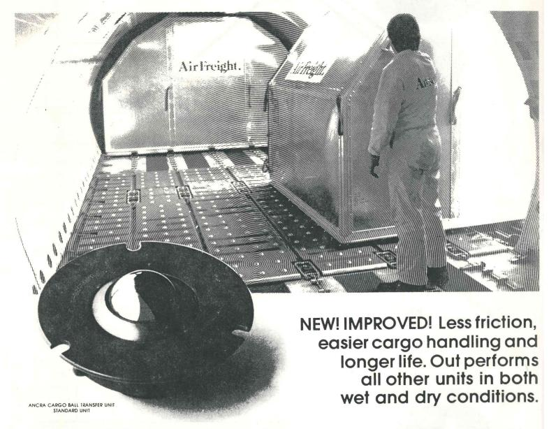
This new omnidirectional ANCRA Ball Transfer Unit moves cargo with less effort, thus reducing loading and unloading time. This light weight rugged unit also carries heavier loads and lasts longer. The secret is ANCRA's patented design that incorporates 25% MORE ball bearings. ANCRA once again has set the standards... for more information contact:
