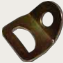
49917-10 1", 45 degree Heat treated, Zinc Plated Gold Chromate Finish. WLL: 1,000 lbs./450 kg. Weight: .10 lbs./05 kg.
