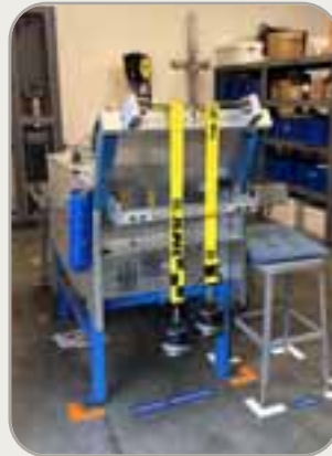
ABRASION TESTER – Webbing samples are abrasion tested per ASTM D67070-097, then load tested for its ability to withstand accelerated wear.
